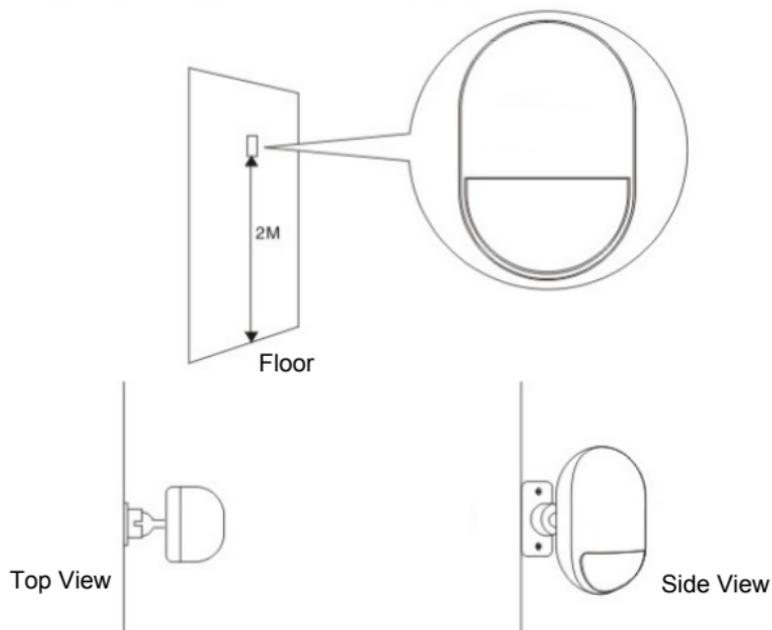
Fix the detector on the bracket, and change the detecting angel and distance through adjusting the installation height and the bracket. The installation height is suggested to be 2 meters high from ground.
