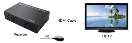
9. If want to control the source, you can use the remote control of source device to send commands subject to IR on the Receiver back to the source to navigate, select and playback the content stored on your source at the far-end device HDTV side.
