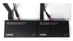
**Step 8:** Connect power of the Sender and Receiver (1,2,3,4), then connect HDMI cable to the "INPUT" of the Sender to HDMI sourcing device and the "OUTPUT" of Sender (1,2,3,4) to the display or TV.
