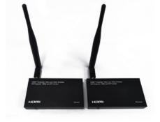
Step 2: By pressing "RESET" button first, the Sender will be connected with power until the Status Led flashes frequently. Then it will take approximately 7s from power on to enter matching mode. The 1.2.3 or 4 Receivers follow the same steps as the Sender.
