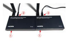
**Step 3:** When the Status Led of the Receiver (1,2,3,4) flashes frequently, it means it entered the matching mode.
