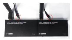
**Step 8:** Connect power of the Sender and Receiver (1,2,3,4), then connect HDMI cable to the "INPUT" of the Sender to HDMI sourcing device and the "OUTPUT" of Sender (1,2,3,4) to the display or TV.
