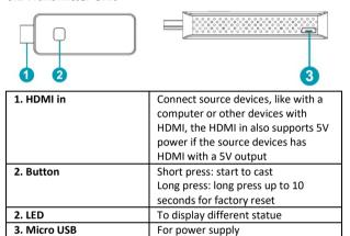
**Remark:** if the source device has a HDMI with 5V power output, then there is no need to connect an USB cable for power.
