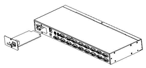
5. After pushing the IP module to the bottom, fix the IP module with the screws of the two fixed brackets that were removed before.
