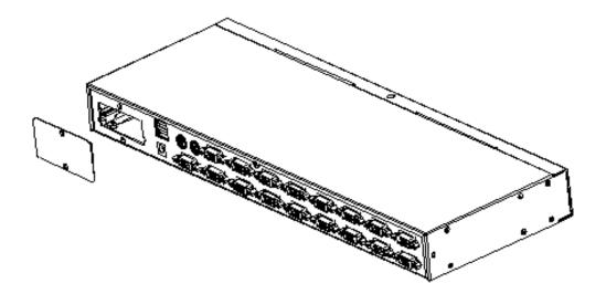
4. Remove the extended IP module and gently push it into the groove of the module cavity as shown.
