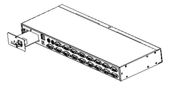
6. After the IP module is installed, before accessing the network cable to enter the switching device, follow the instructions of the IP module to install the related software and configure the network IP address of the device. After the setting is completed, you can access your network to log in. use. (For details, please refer to the product instruction manual of the IP module.)
