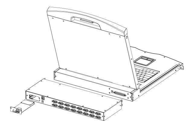
1. Locate the rear of the unit and install the outer bracket of the expansion slot. You need to prepare a screwdriver as a tool for disassembly and installation.
