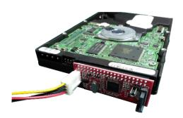
3. Connect the 4 PIN power cable to your IDE device.
