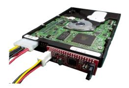
4. Connect a SATA cable to IDE to SATA adapter and remember to plug the other connector of the cable to your computer.
