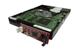
Plug the 4 PIN power cable to IDE to SATA adapter.
