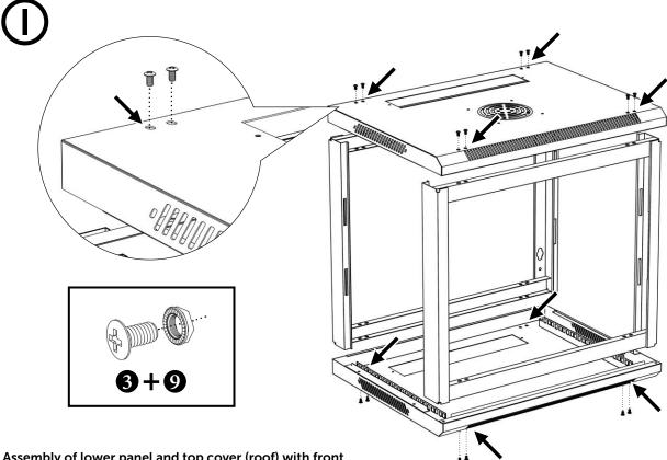
Assembly of lower panel and top cover (roof) with front and rear structural frames.
