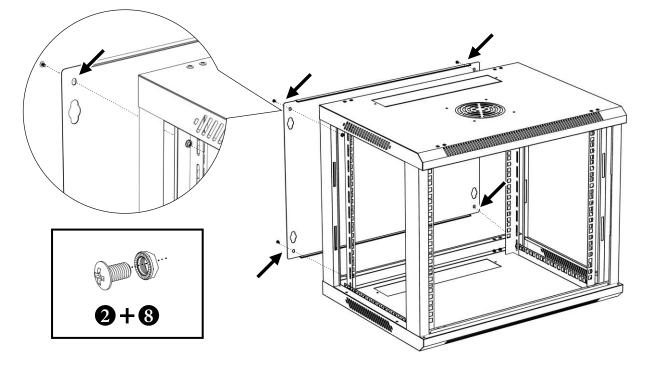
Installing the Side Panels, Side Panel Latches, and Front Door Hinges.
