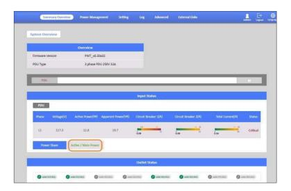
**Step 9:** The related log and trap will be recorded on the **Log** of **Event Log** webpage and NMS. The log and trap will be "Information: Inlet (PDU:1) Active/Backup Power change to Active/Main Power".
