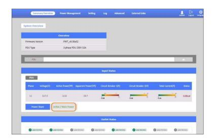
**Step 3:** When PDU A has utility power fail, the status of power share will display **Active/Backup Power** on the **System Overview** webpage.
