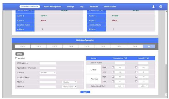
DIGITUS® PDU supports 8 EMD sensors in cascade each one with 2 digital inputs to set 2 alarms for each EMD 31 sensor. There are 3 options(Normal Open/Normal Close/Disable) of the EMD sensor. If you set "Normal Open", the EMD sensor will become "Warning"(Yellow light) when closed.
