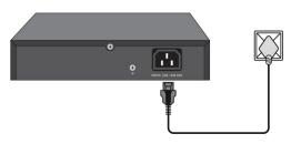
**Warning:** Do not turn on the power switch before power cables are connected. Power surge may cause damage to the Switch.
