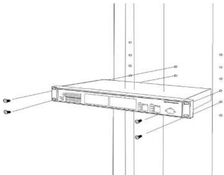
Figure 1 Locating a Mounting Bracket
