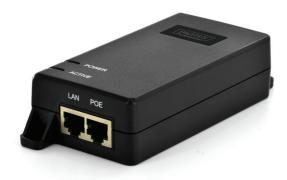
Manual DN-95103-2 DN-95103-2, it is the single-port 30w PoE injector with detection chip inside. The output voltage is 55VDC/550mA, output power 30W. It fully comply to IEEE802.3at standard, and only supply power for PoE standard PD such as, indoor wireless AP, network camera, IP phone...etc.
