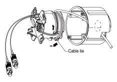
**5** Place back faceplate, remove protective dust cap from cable, insert the cable to FO adapters on fiber module
