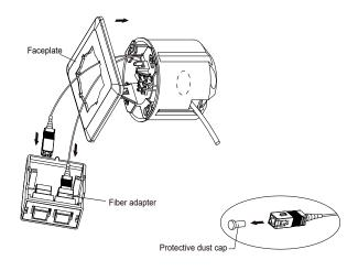
Insert fibers into wall box, cut and keep ca. 150mm pigtail fibers for splicing and splice them according to the instruction of the splice unit used.
