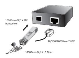
Figure 5-2: DN-82140 Installation
