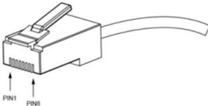
This cable is used to connect the console port of the switch to the external monitoring terminal. One end of the RJ45 eight-pin
