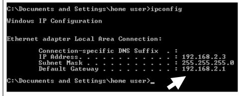
4. Input 'ipconfig', then press 'Enter' key. Please check the IP address followed by 'Default Gateway' (In this example, the IP address of router is 192.168.2.1)
