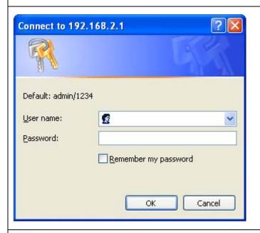
5. Start the web browser and input the IP address of wireless router in address bar, and the following message should be shown. Please input user name and password, then click 'OK' to access web management interface of wireless router.
