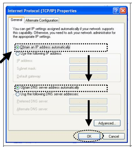
2. Select 'Obtain an IP address automatically' and 'Obtain DNS server address automatically', then click 'OK'.
