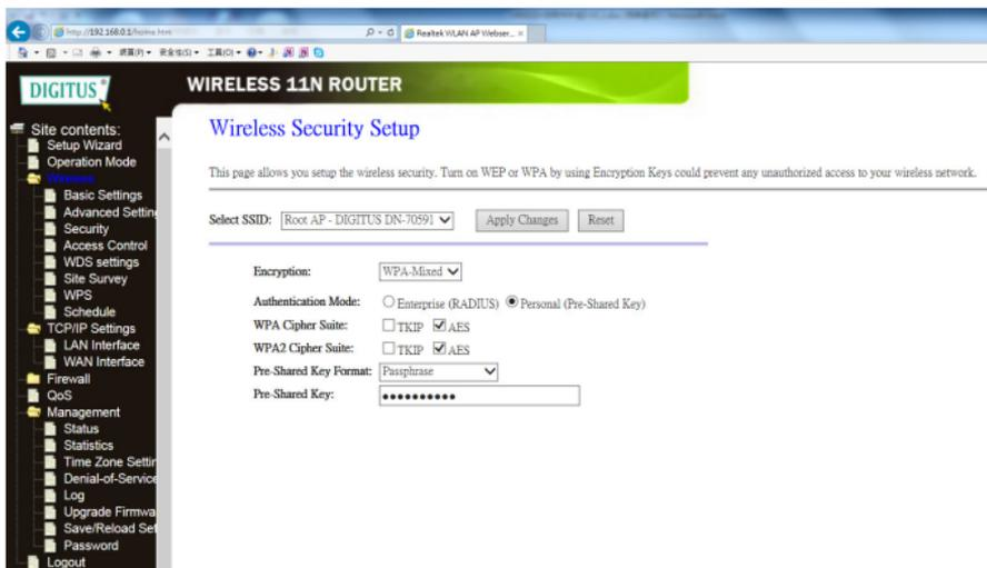
The screenshot shows the web interface of a DIGITUS WIRELESS 11N ROUTER. The page title is "Wireless Security Setup". A navigation menu on the left lists various settings, with "Wireless" expanded to show "Wireless Security". The main content area contains the following fields and options:
