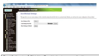
Reset Settings to Default Click this '**Reset**' button to remove all settings you made, and restore the configuration of this router back to factory default settings
