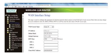
If your ISP provides the DHCP service, please choose 'DHCP Client', and the Router will automatically get IP parameters from your ISP. This page displays the WAN IP parameters assigned dynamically by your ISP, including IP address, Subnet Mask, Default Gateway, etc.
