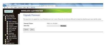
After a firmware upgrade file is selected, click '*Upgrade*' button, and the router will start firmware upgrade automatically. The procedure may take several minutes, please wait for this process to complete.
