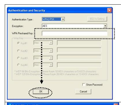
3. If the wireless access point uses encryption, you have to input WEP passphrase or WPA preshared key. Please ask the owner of the wireless access point you want to connect, and input the correct passphrase / preshared key here, then click 'OK'. If the value you inputted here is wrong, you will not be able to connect to wireless access point.
