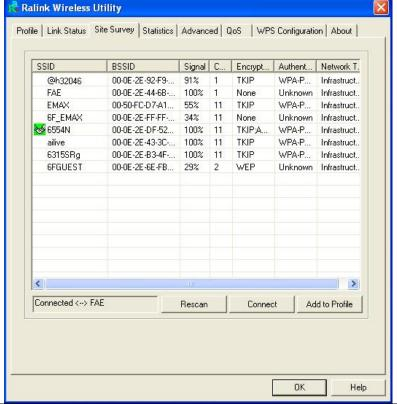
4. If the wireless access point is successfully connected, you'll see a 'Connected' message displayed at the lower-left corner of wireless configuration utility window. Click 'OK' to exit.
