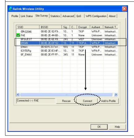
2. Configuration utility will scan for wireless access points automatically, and all found access points will be displayed. Please select an access point you wish to connect, and click 'Connect'.
