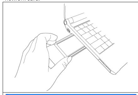
1. Please insert the wireless network card into an empty PCIe ExpressCard slot of your computer. You can insert the card when the computer is power off or on.
