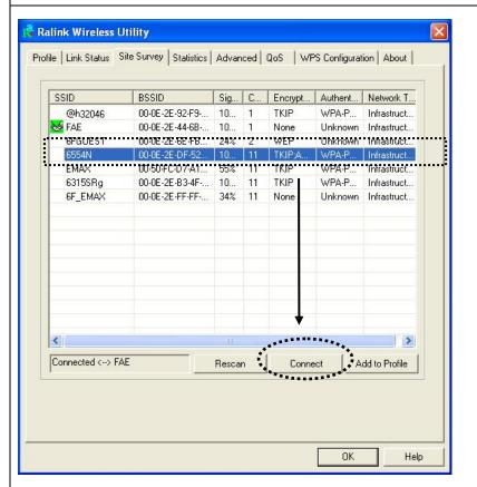
2. Configuration utility will scan for wireless access points automatically, and all found access points will be displayed. Please select an access point you wish to connect, and click 'Connect'.
