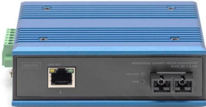
**Front panel:** The yellow LED on the RJ45 port is the LINK light, which is on when the connection is established and the data transmission is flashing. The green light on the RJ45 port is PoE light, which is only on when the switch port is supplying power to the PD devices (PoE DN-652104-1 only) Link/Act is green color when optical connection. Power indicator light is on when connecting with Power.
