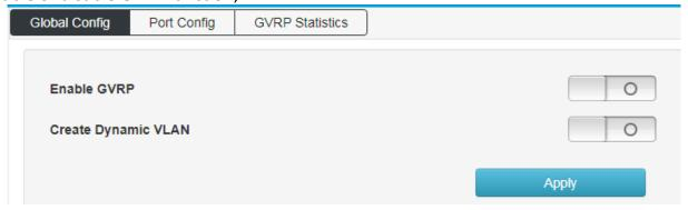
Apply the enabled GVRP function to the designated port and configure its timer;
