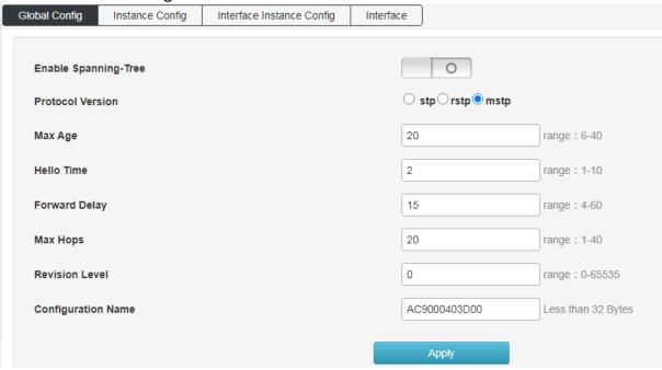
Instance configuration: configure MSTP instance, Set the mapping Vlan for multiple spanning trees
