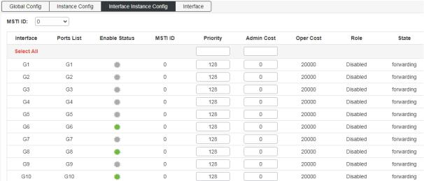
Interface configuration: Configure the ports enabled for spanning tree protocol and the enabled ports for BPDU packets;
