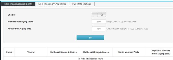
MLD Snooping VLAN configuration: Configure static multicast VLAN;
