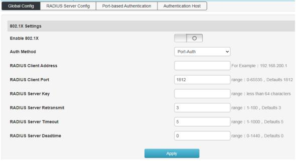
Figure 4-10-2 RADIUS Server Config interface
