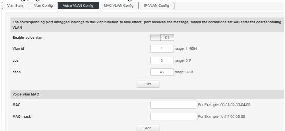
When the voice VLAN feature is enabled, the Access port can carry IP voice traffic from IP phones. When the switch is connected to a Cisco IP phone (such as a Cisco 7960 IP phone), the voice traffic sent by the IP phone has three layers of IP priority. And the CoS value of the second layer, both of these two values are set to 5 by default. For IEEE 802.1Q or IEEE 802.1p tagged traffic, the default COS value is untrusted.
