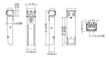
LC connector, Gigabit, 20km Single mode, Single fiber (DN-81020 and DN-81021)
