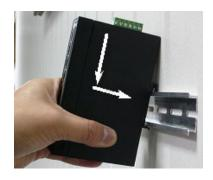
**Step 2:** Check the DIN-Rail is tightly on the track.
