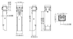
LC connector, Gigabit, 20km Single mode, Single fiber (DN-81020 and DN-81021)
