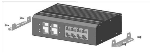
Figure 2-2 Install hangers diagram
