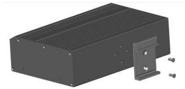
Figure 2-1 Install Din-rail hangers diagram
