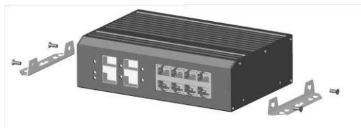
Figure 2-2 Install hangers diagram
