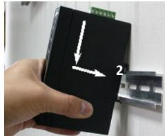
Figure 5: Install Industrial Equipment in DIN-Rail mount.
