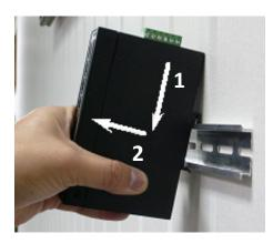
Figure 7: Remove Industrial Equipment in DIN-Rail mount.
