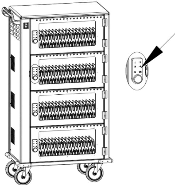
2. By tablet number, Place the tablets one by one into the tablet rotation slot with the corresponding number.
