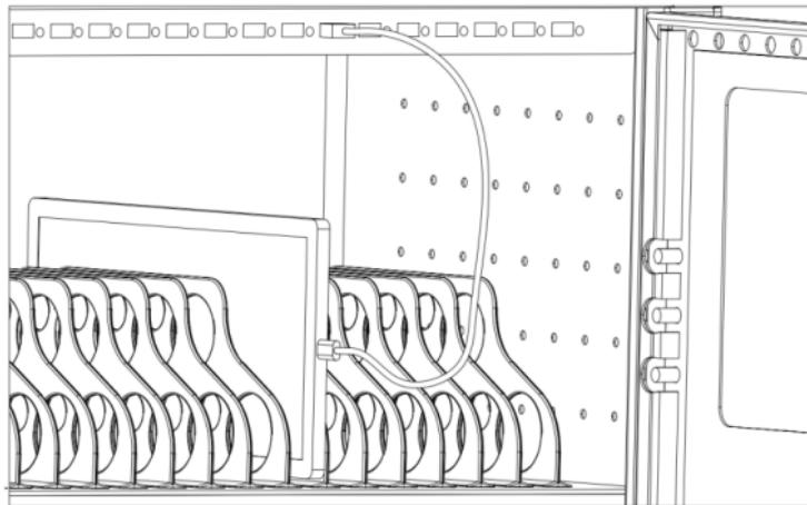
4. After the connection is completed, Lock the cupboard door, Plug the charger into the mains outlet and prepare to start charging.
