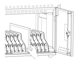
3 The two ends of the USB cable are connected to the charging /HUB port on the device and the tablet port respectively.
