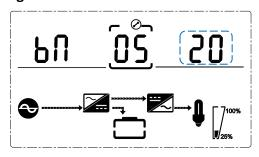
Battery quantity setting (Note: Inside the broken-line is the flashing part.)
