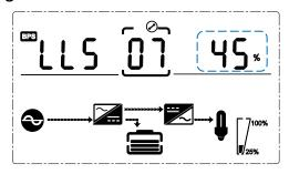
Bypass voltage lower limit setting (Note: Inside the broken-line is the flashing part.)
