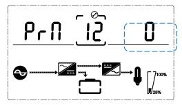
Parallel redundancy quantity setting
