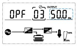
Frequency setting (Note: Inside the broken-line is the flashing part.)
