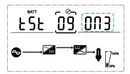
When choosing On3, UPS can transfer to Battery Mode automatically per 30 days. And the Battery Self-test Time is EOD.
