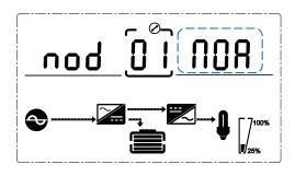
Mode setting (Note: Inside the broken-line is the flashing part.)
