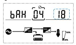
Battery capacity setting (Note: Inside the broken-line is the flashing part.)
