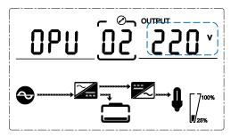
Output voltage setting (Note: Inside the broken-line is the flashing part.)
