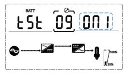
When choosing On1, UPS can transfer to Battery Mode automatically per 30 days. And the Battery Self-test Time is 10 seconds.
