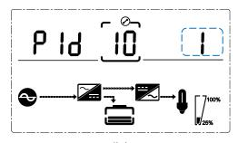
Parallel ID setting (Note: Inside the broken-line is the flashing part.)
