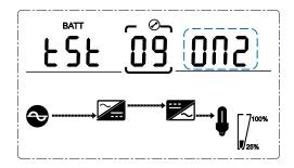
When choosing On2, UPS can transfer to Battery Mode automatically per 30 days. And the Battery Self-test Time is 10 minutes.
