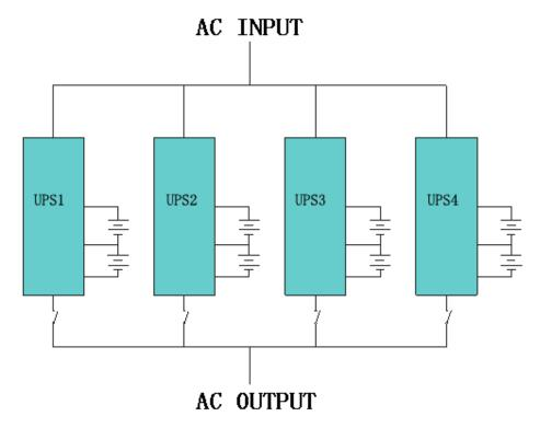
Make sure each UPS input breaker is in "off" position and there is no any output from each UPS connected. Battery groups can be connected separately or in parallel, which means the system itself provides both separate battery and comman battery.
