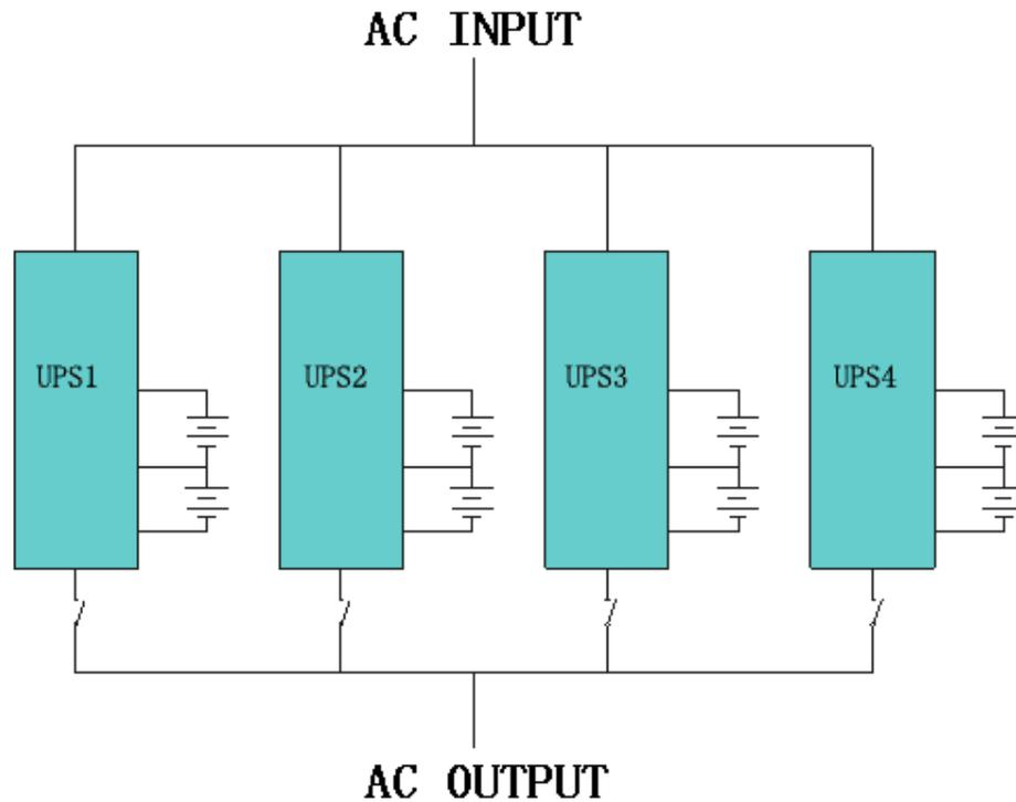
Make sure each UPS input breaker is in “off” position and there is no any output from each UPS connected. Battery groups can be connected separately or in parallel, which means the system itself provides both separate battery and common battery.
