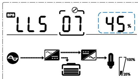
Bypass voltage lower limit setting
