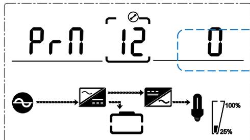
Parallel redundancy quantity setting
