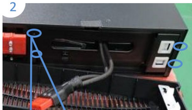
Fix battery cover by screws
