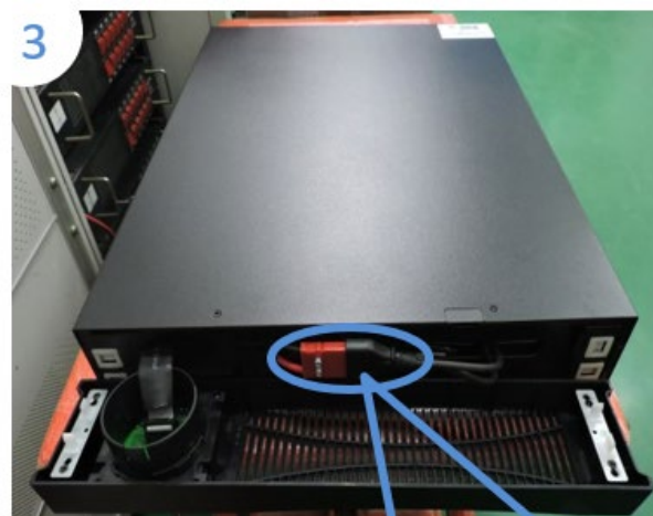
Interlock the battery wire and combine wire terminal.
