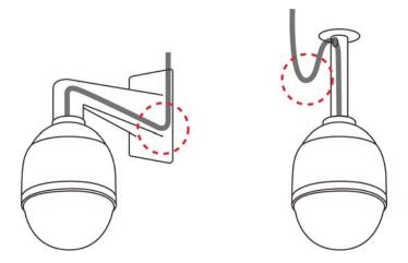
• The cable entry hole of the outdoor mounting kit (indicated in the figure below) needs to be sealed to avoid water from entering the camera.
