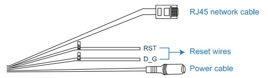
Note: The regulated power adapter is DC12V (600mA) to operate this device.
