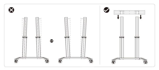
If the columns are not properly aligned, the mounting plate may fail to attach to the columns. Follow the steps below to re-assemble the columns.
