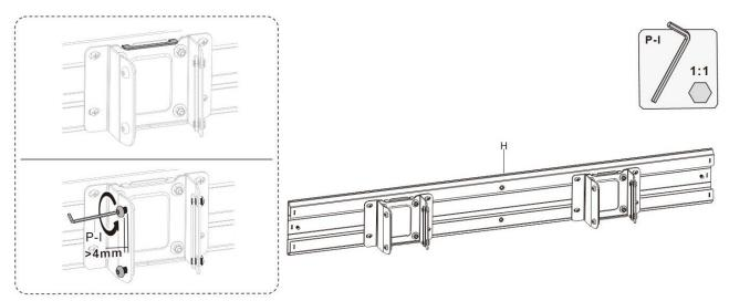
Loosen the screws to leave a gap over 4 mm
