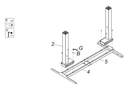
Using screws (B) to connect the lifting column (2) with the left supporting beam (4) and the right supporting beam (5), and tighten them with the allen key (G)
