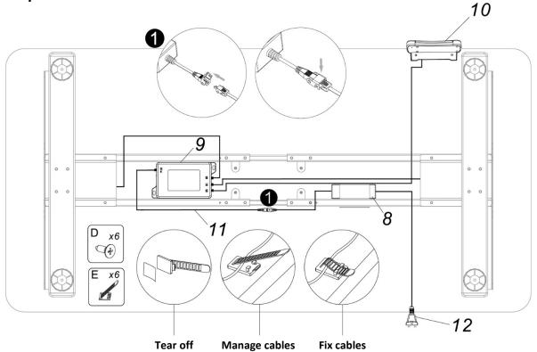
Fix the cables to the tabletop with cable management (E), and then use screw (D) to fix the cable management (E) to keep the desk cables organized.
