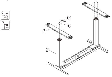
Connect the feet (1) and the lifting column (2) with screws (C) and tighten them with the allen key (G)
