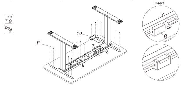
• Fix the tabletop with screws (F), and then to fix the control box (9) on the tabletop with screws (F). The handset (10) is fixed on the tabletop with selfowned screw and insert the adapter into the adapter arm.
