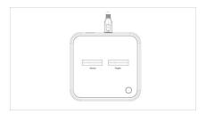
Pressing clone button for several seconds, till clone LED light 25% flash
