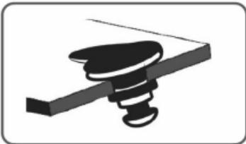
A 3D illustration shows the SSD being pushed into the bracket. A black, dome-shaped silicone pad is positioned on top of the SSD to ensure it is seated correctly and held in place. |
