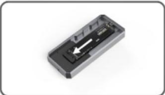
The M.2 SSD is shown inserted into a metal mounting bracket. A white arrow on the bracket points to the left, indicating the direction to push the SSD into the slot.                |
