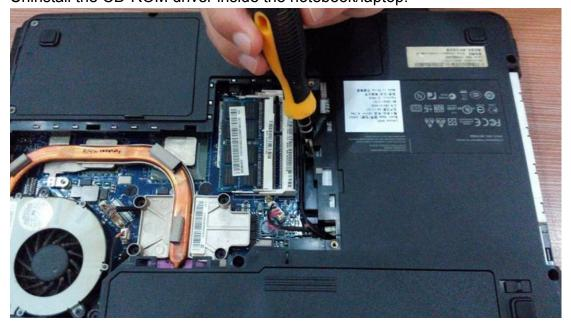
Once remove the CD-ROM driver, please check the thickness of the driver which is 12.7mm or 9.5 mm. In order to pick up the suitable 2nd HDD Caddy, it has to make sure the connector of CD-ROM driver is for SATA or IDE.
