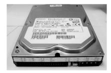
3) Connect IDE cable and 4 sin power adapter cable on your hard drive.
