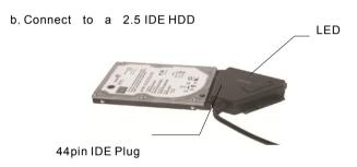
For a 2.5 SATA HDD or IDE HDD, plug directly the SATA connector or the 44pin connector into the appropriate ports on the rear of the HDD, and plug the USB signal/data plug (Black) into USB port of PC.
