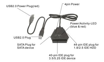
Note: For 3.5/5.25 IDE devices, please plug in a 5V/12V power supply (not included) to appropriate port on the back side of HDD or DVD, so that the PC power switch (on/off) can't control the current to HDD or DVD. If you want to cut off the current to HDD or DVD, then you need to plug out the power plug from 3.5" IDE HDD or 5.25 DVD devices.
