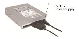
For a 5.25 CD/DVD device, plug directly the 40pin connector into the appropriate ports on the rear of the CD/DVD device, and plug the USB signal/data plug (Black) into USB port of PC, then plug the 4-pin plug of the power supply to the 4-pin power jack (for IDE CD/DVD direct plug in CD/DVD power connector), and the other end plug to power source.
