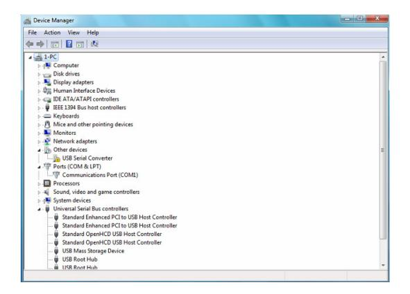
Step 6: Right click on the other device to bring up a menu as shown below. From the displayed menu select "Update Driver Software..." This then displays the option for an automatic search or a manual search.
