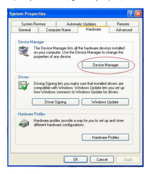
Step 20: Select "Device Manager" in the "Hardware" of the interface "System Properties", click it, you can see the hardware devices installed on your computer, please refer to the following chart:
