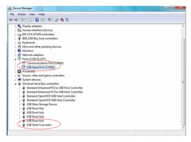
This time the Device Manager does not have a USB <->Serial Cable entry under Other Devices but does show entries under Universal Serial Bus Controllers and Ports (COM & LPT). The above screen shot displays a correct installation. The device is now ready to use on COM3.
