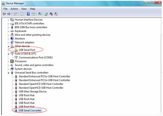
The Device Manager will still show a device under Other Devices but in addition to this there is a new entry under Universal Serial Bus Controllers indicated in the screenshot above as the USB Serial Converter. This indicates the bus layer of the driver is installed. Installing the Virtual Com Port layer of the driver is almost a repeat of the last few steps.
