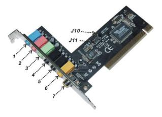
The rear panel of this 7.1 Channel PCI Sound Card has the following jacks:
