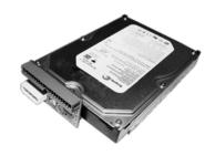
Plug the IDE cable to SATA 150 to PATA Converter and please remind the direction of IDE PIN.
