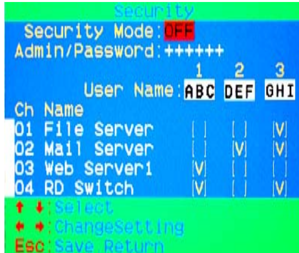
Figure 27: Security setup main window
