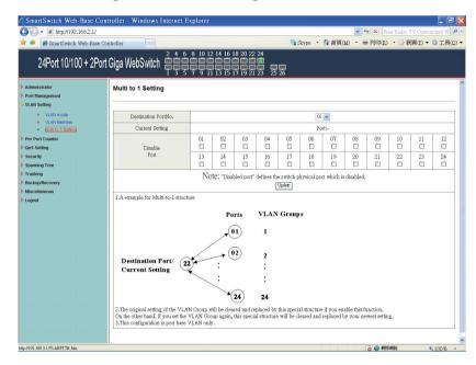
This is a special design for easily setting the switch VLAN into "VLAN Per Port".
