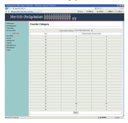
You can read the transmitting and receiving packet of the connecting port.
