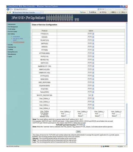
You can set QoS mode of per port by different bases. TCP/UDP > TP TPS/DS > 802.1P > Physical port
