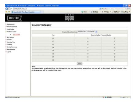
You can read the transmitting and receiving packet of the connecting port.
