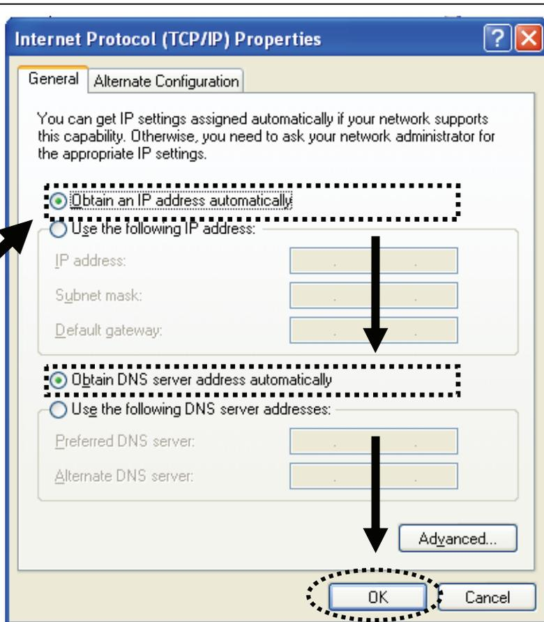
3. Отметьте "Obtain an IP address automatically" и "Obtain DNS server address automatically" после чего нажмите "OK".
