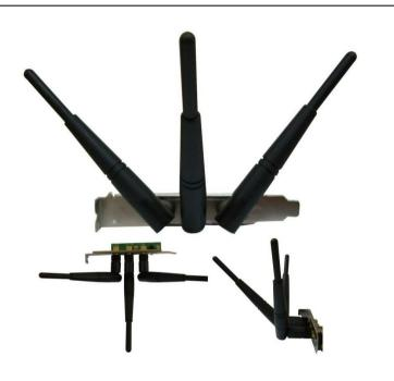
2. Install all three antennas on the wireless network card, and make sure the antennas are securely installed. To improve radio reception, please adjust antennas to the position shown in the left picture.
