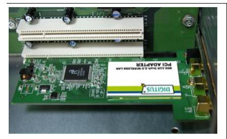
1. Turn off your computer, and remove the case as required so you can see PCI expansion slots (PCI slots are usually colored as white), and then insert the PCI wireless network card into any available the PCI slot.
